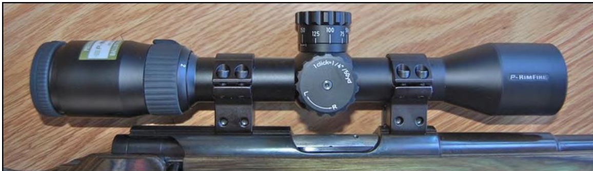
Rimfire scope with semi-target turrets, Nikon P-Rimfire 2-7 x 32mm, Hawke rings mounted in dovetail.
