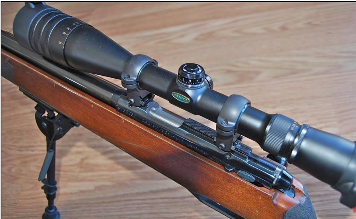
Weaver 4-16 x 42mm with semi-target turrets, AO (adjustable objective), mounted in Burris Signature Zee rings on Weaver bases in dovetail - note plastic inserts in rings.
