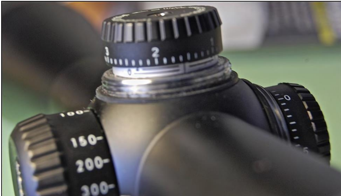
Target turrets: SF on left, windage on right, elevation on top - note the lines below the movable knob which indicate number of revolutions, a great feature to have.
