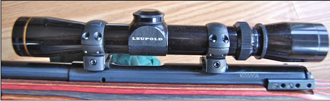
Leupold Rimfire 2-7 x 28mm in Weaver rings on Weaver bases installed in drilled and tapped holes in receiver.
